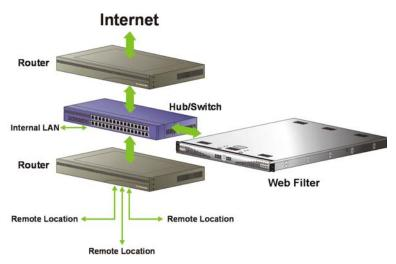
Fig. 1:1-3 Router mode diagram
