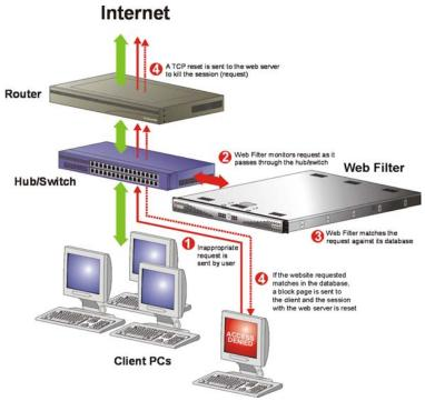
Fig. 1:1-1 Pass-by filtering diagram
