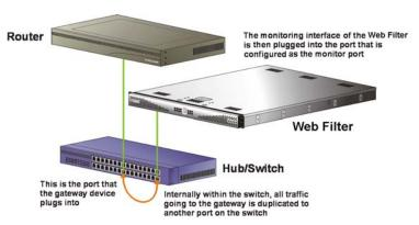
Fig. 1:1-2 Invisible mode diagram, with port monitoring
