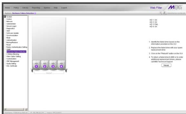
Fig. 2:1-62 Hardware Failure Detection window, 500 series model
