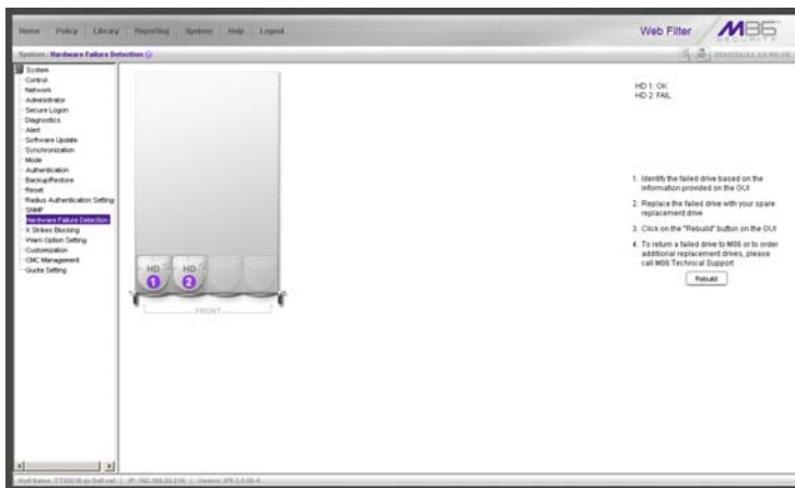
Fig. 2:1-62 Hardware Failure Detection window, 500 and 700 series
