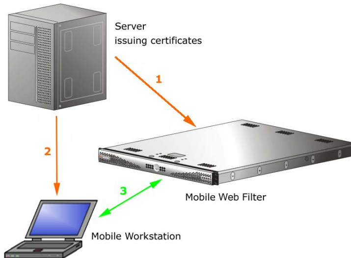
Fig. 2-2 Enterprise PKI mode server flow
