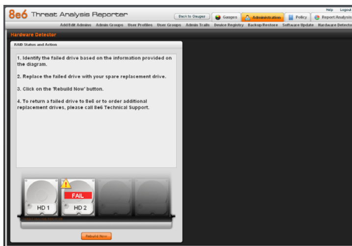
Fig. 4.6-2 Hardware Detector, hard disk failure
