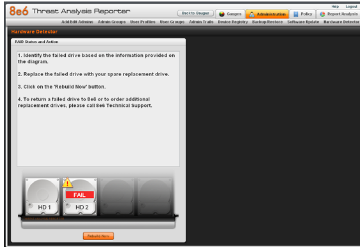
Fig. C-2 Hardware Detector panel, failed hard drive detected
