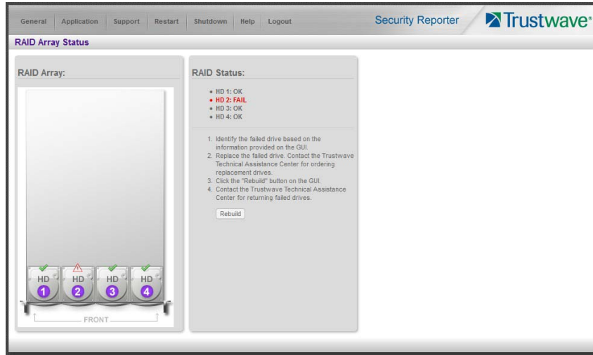
Figure 10: RAID Array Status screen, 505 IBM model
