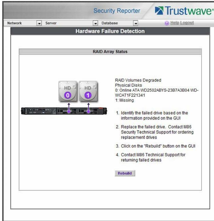
Figure 6: Hardware Failure Detection screen, 705 or 735 IBM model
