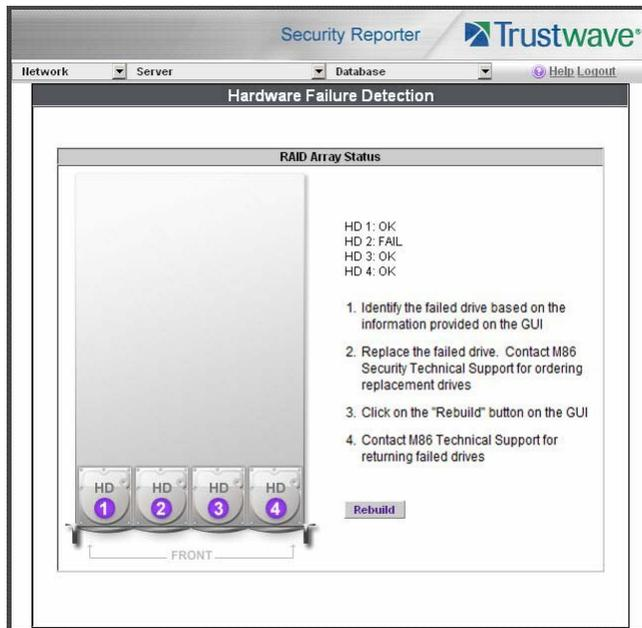
Figure 9: Hardware Failure Detection screen, 505 IBM model
