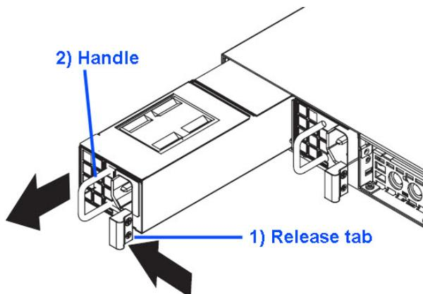
Note that an audible alarm sounds and the LED is unlit when the power supply module is disengaged. Replace the failed power supply with your spare replacement power supply module. The alarm will turn off and the LED will be a steady green when the replacement power supply module is securely locked in place.
