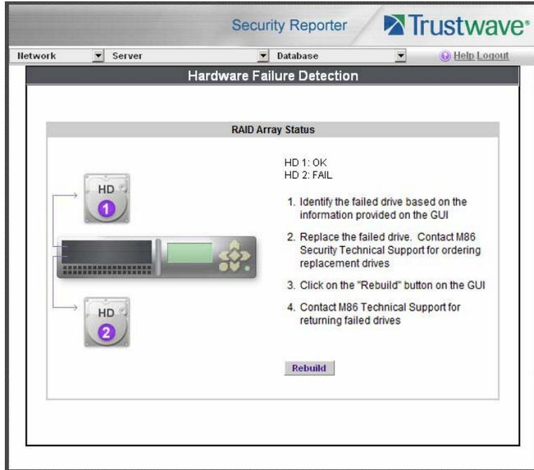
Figure 4: Hardware Failure Detection screen, 500, 700, 730 model
