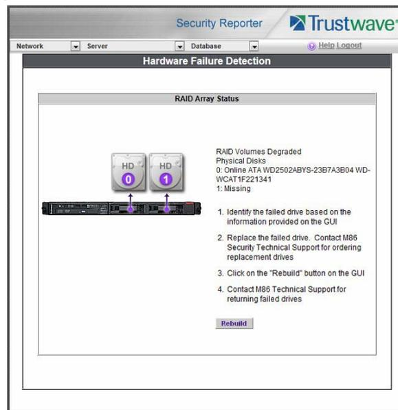
Figure 10: Hardware Failure Detection screen, 705 or 735 IBM model
