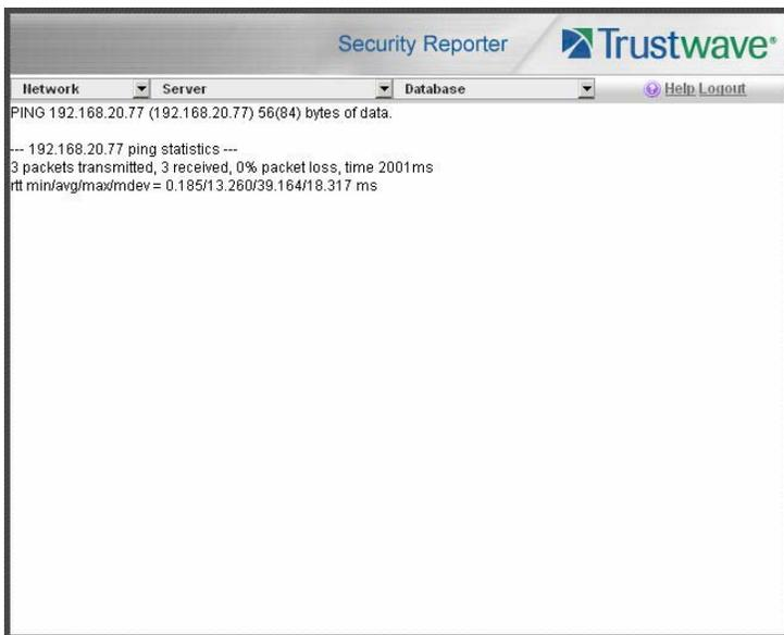
As indicated by the results for the sample entry, the server at 192.168.20.78 was able to communicate with the machine at the IP address 192.168.20.77. The statistics show that three (3) data packets were transmitted by the server, and three (3) packets were received by the designated machine, for a total of zero (0) percent packet loss.
