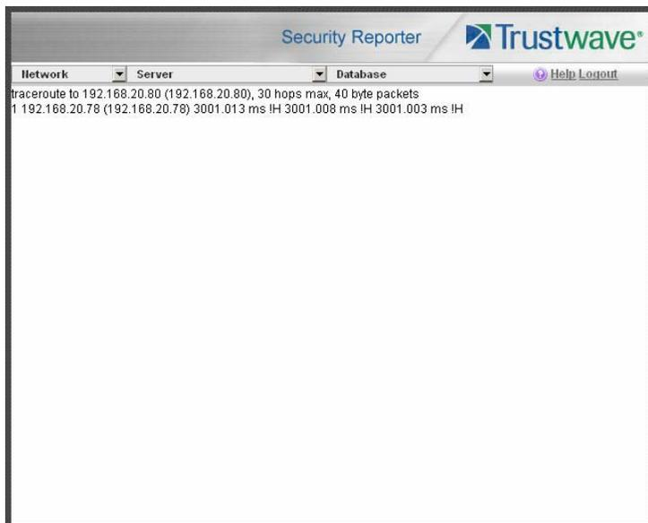
As indicated by the results for the sample entry, the packet made 30 hops. For each line in the report, the hop number displays, followed by the IP address or hostname; the IP address in parentheses; and the maximum, minimum, and average response time in milliseconds.
