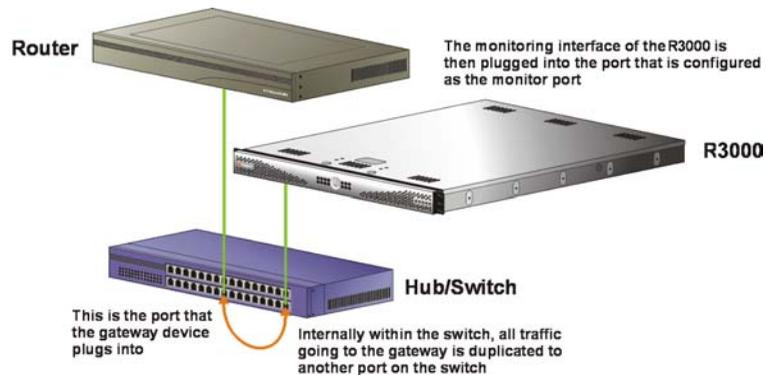
*Fig. 1:1-2 Invisible mode diagram, with port monitoring*
