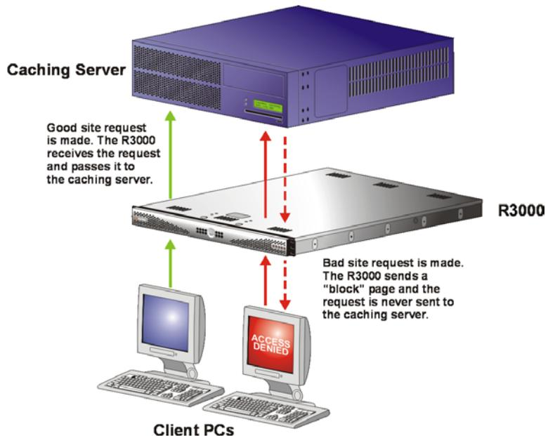
Fig. 1:1-4 Firewall mode diagram, with firewall and cache setup
