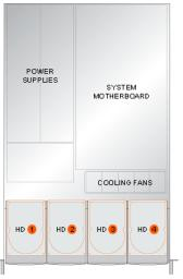
Fig. C-1 ER RAID Server components
