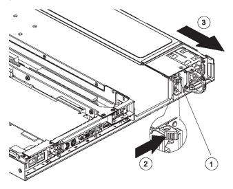
Note that an audible alarm sounds and the LED is unlit when the power supply is disengaged. Replace the failed power supply with your spare replacement power supply. The alarm will turn off and the LED will be a steady green when the replacement power supply is securely locked in place.
