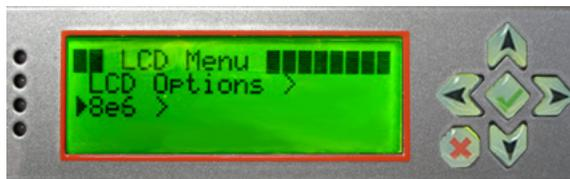
In the LCD panel, an arrow displays to the left of the currently selected menu item. Use the up or down arrow keys to navigate the menu. After making your menu selection, press the checkmark key to accept your selection.
