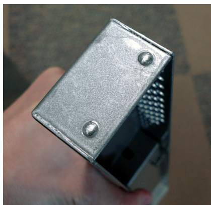
Fig. 2 - Bumps on right end of bezel
