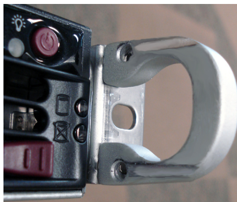
Fig. 3 - Grooves in right U-shaped handle
