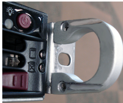
Fig. 3 - Grooves in right U-shaped handle
