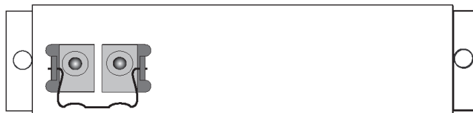
AC power in rear panel of NetOptics 10/100BaseT Tap
