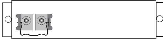
AC power in rear panel of NetOptics 10/100BaseT Tap
