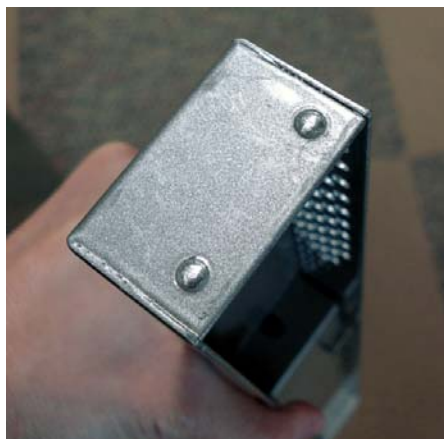
Fig. 2 - Bumps on right end of bezel
