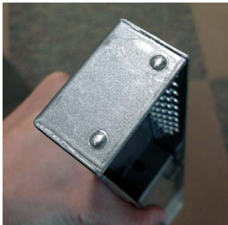
Fig. 2 - Bumps on right end of bezel
