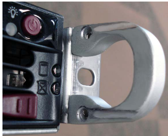
Fig. 3 - Grooves in right U-shaped handle
