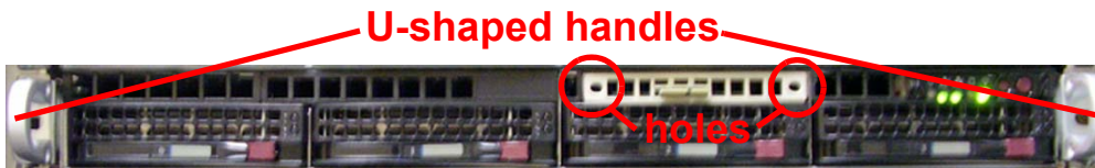
Fig. 4 - Front of chassis with U-shaped handles and holes above third hard drive identified
