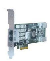
Silicoms Gigabit Ethernet Bypass server adapters include an on board WDT (Watch Dog Timer) controller. The adapters software drivers or software application can write commands to the on board WDT controller. The adapters software drivers, WDT controller and the Bypass circuitry provide an interface that control and manage the mode of the adapter.
