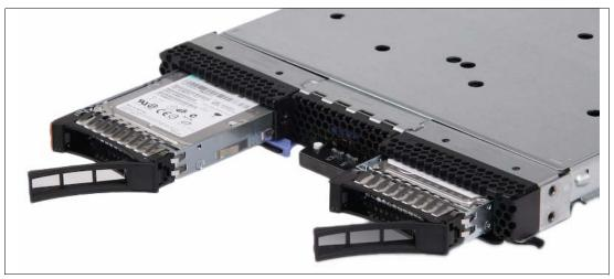
Figure 7 The HS22 showing the front hot swap disk drive bays
