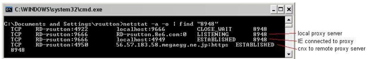
Netstat output showing Ultrasurf's TCP connections
