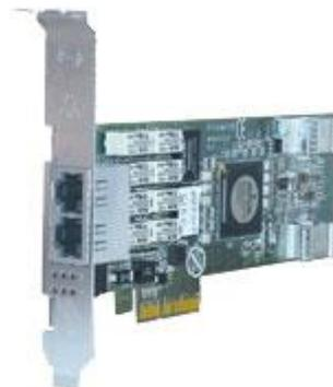
Silicom's Gigabit Ethernet Bypass server adapters include an on board WDT (Watch Dog Timer) controller. The adapters software drivers or software application can write commands to the on board WDT controller. The adapters software drivers, WDT controller and the Bypass circuitry provide an interface that control and manage the mode of the adapter.
